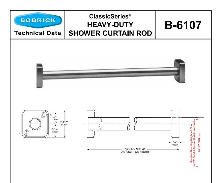
**Curtain Rod** — 18-8, Type-304, 20-gauge (1.0mm) stainless steel tubing with satin finish. 1" (25mm) outside diameter. Available in lengths 36" (915mm) up to 72" (1830mm).
